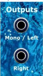
For a rich-sounding *mono* output, just use the **Mono / Left** output socket by itself, with the **Right** socket disconnected.
