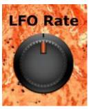
The original Small Stone, in common with many early stomp-box phasers, gave you very limited control over parameters. In fact, all you can do is tweak the sweep cycle rate of its internal triangle wave LFO. This limitation has been carried forward into Kleiner-Kiffer. The internal LFO covers roughly the same frequency range as the original – from 0.04 Hz (25 seconds per cycle) up to 12 Hz.
