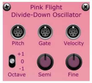
Pink Flight connects to the **Poly Pitch**, **Poly Gate** and **Poly Velocity** sockets on the Voltage Modular **Poly Sources** panel. You can also set the number of polyphonic voices (from 1 to 16) through this panel. If the velocity socket is disconnected, each voice will sound at full intensity when triggered.
