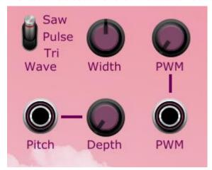
Pink Flight offers three waveform types - sawtooth, triangle and variable pulse (with Pulse Width Modulation).
