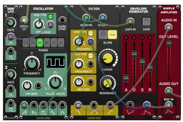
When the envelope voltage is at OV, the Audio Out will be silent, regardless of the setting of the Out Level slider.
