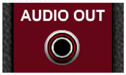
The Audio Out socket is where the module sends its processed Audio In signal, after being attenuated by the Out Level control and the Env In control voltage.
