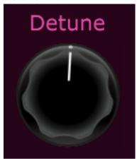
The Detune knob sets the linear frequency difference between Osc 1 and Osc 2. The frequency difference (in absolute Hz) is constant, regardless of the musical pitch of the oscillators. This differs from most other voltage controlled oscillators, where the absolute frequency difference increases as the pitch rises. In standard VCOs, the frequency *ratio* between two oscillators is kept constant.
