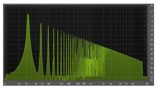
Note that the fundamental frequency (at 32 Hz) is 6 dB higher than it is in the "Norm" setting.
