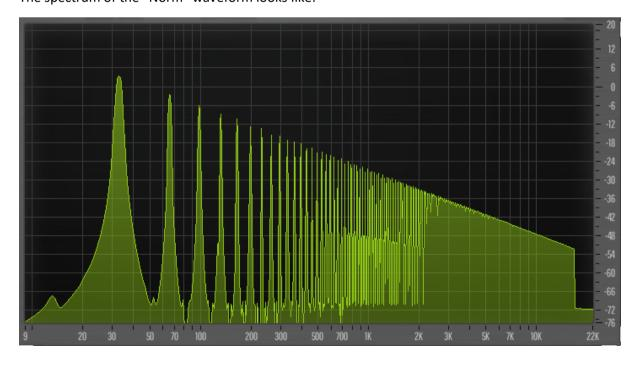
In the "Cut" position, the oscillator will output a standard falling sawtooth waveform with its fundamental component removed:
