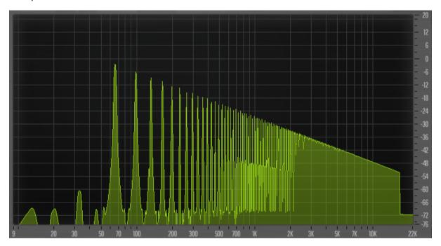
Note that the fundamental frequency (at 32 Hz) is missing.
