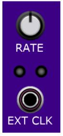
The module works by sending out note-on messages for all the keys stored in Bank A for a short duration, then note-off messages. Then, the Bank B notes are played for a short duration, and the cycle repeats. It can be thought of as a two-stage arpeggiator which can play block chords on each step.
