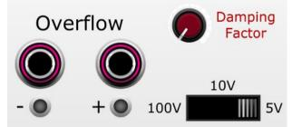
The Integrator can operate within three output voltage ranges: +/- 5V, +/- 10V and +/- 100V. Choosing the +/- 5V range ensures that the output can be used as an audio signal within the Voltage Modular environment. The 10V and 100V ranges are provided to help avoid 'runaway' positivefeedback situations.
