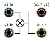
Bipolar DC voltages and AC voltages are allowed as inputs, and the output sign follows the inputs over all four quadrants:
